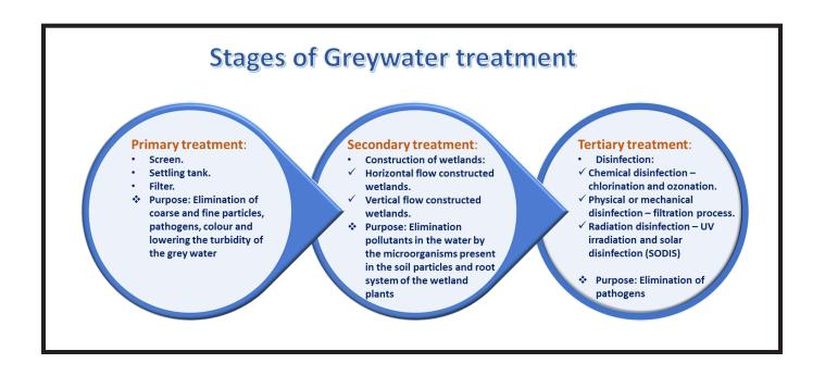
The basic three stages of treatment involve primary, secondary, and tertiary treatment. These stages sequentially treat the greywater and make it viable for reuse applications. The figure below depicts the major treatment stages with their related processes.
